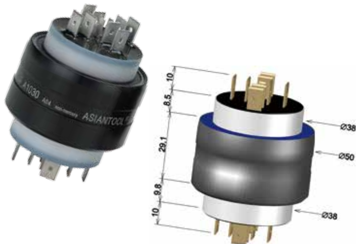
A1030 NM (non-mercury) 8poles/30A & 2poles/4A AC250V
