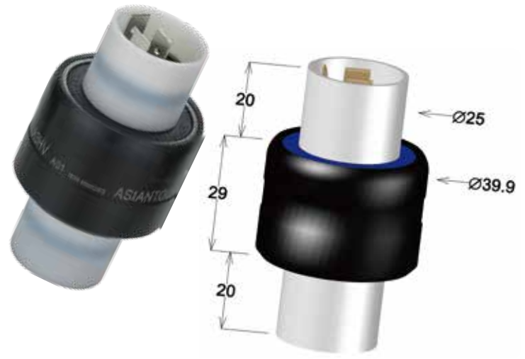
A3HV NM (non-mercury) 3poles/30A/AC500V
